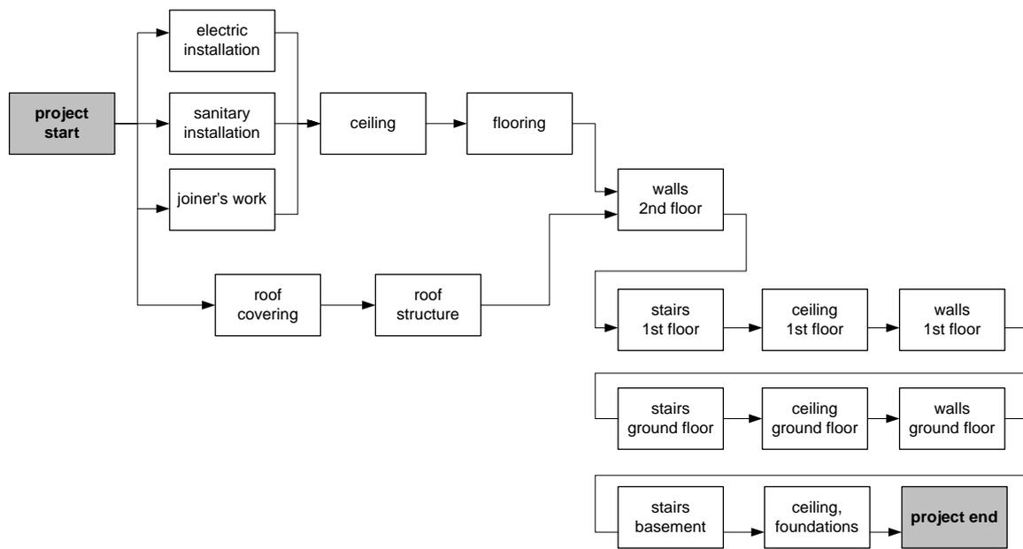
**Fig. 3 Activity-on-node network of a deconstruction project (simplified)<sup>3</sup>**
