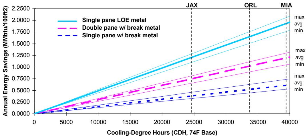
**Figure 1:** Sample Energy Efficient Window Alternatives. Range and average energy reduction when modeled in place of MEC minimally compliant single pane, aluminum frame baseline (JAX = Jacksonville, ORL = Orlando, MIA = Miami).
