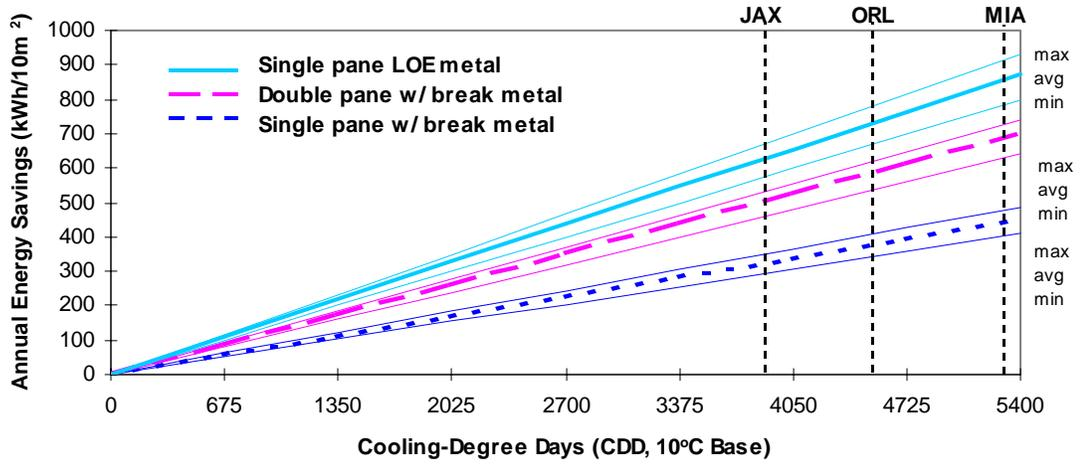
Figure 1. Sample energy efficient window alternatives. Range and average energy reduction when modeled in place of MEC minimally compliant single pane, aluminum frame baseline. JAX = Jacksonville, ORL = Orlando, MIA = Miami. (Grosskopf, 1998)
